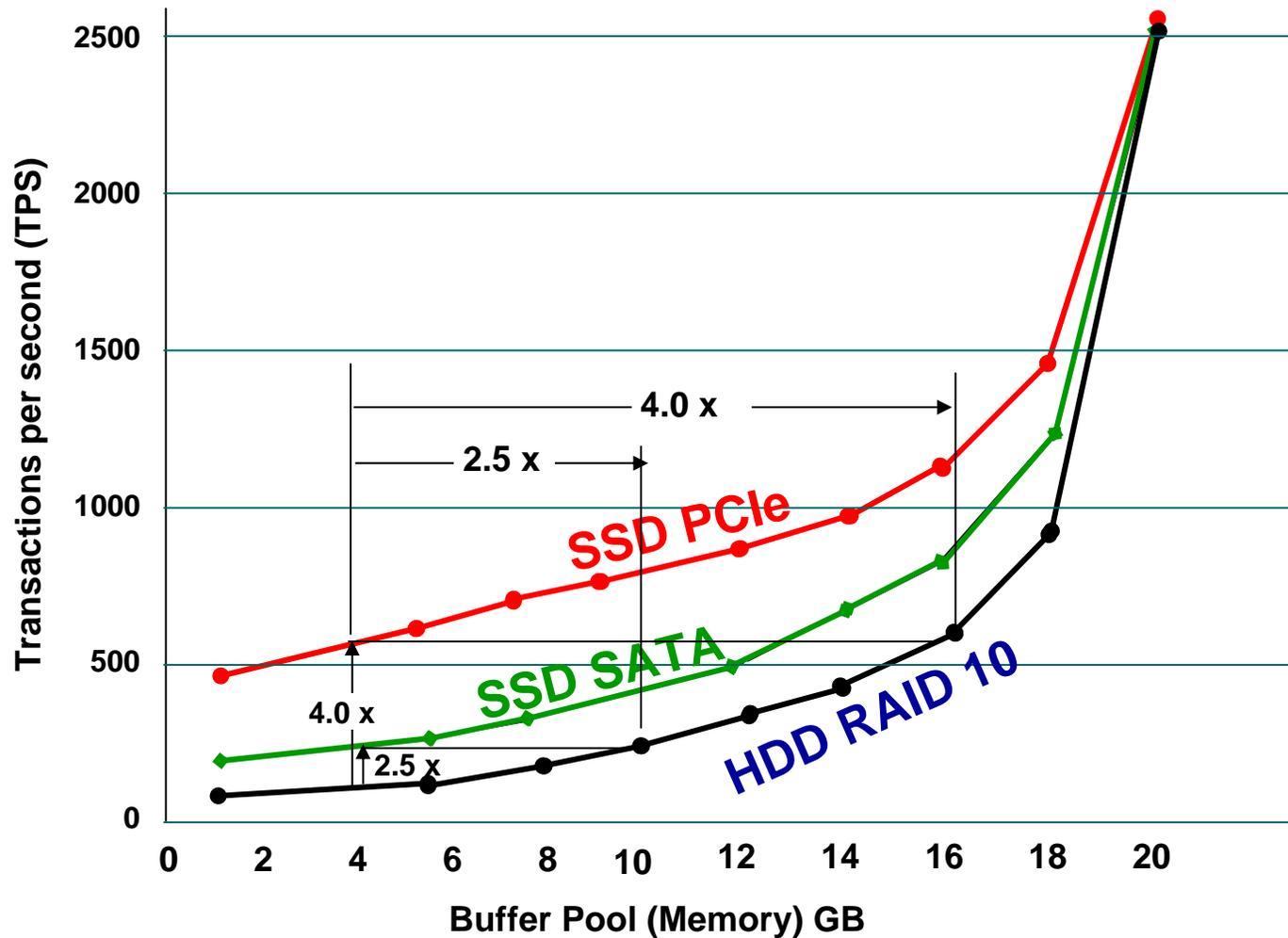
To achieve a certain TPS improvement, its cheaper to deploy SSD vs increased buffer memory (in GB costs) needed with using HDDs alone.
