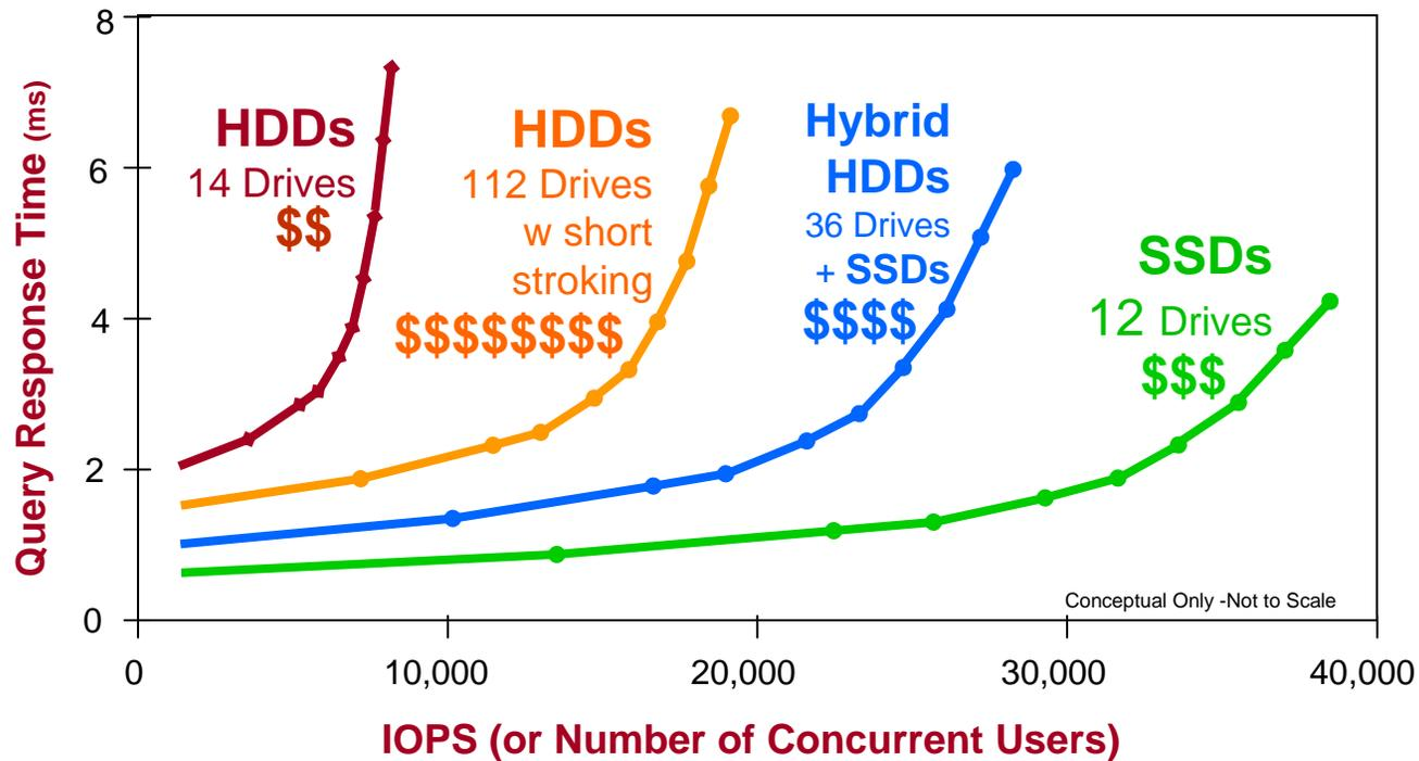
For a targeted query response time in DB & OLTP applications, many more concurrent users can be added cost-effectively when using SSDs or SSD + HDDs storage vs. adding more HDDs or short-stroking HDDs
